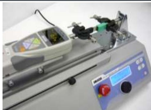
USB connector extraction / insertion (repetition) test
